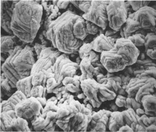
Figure 3 Scanning electron micrograph of \text{Nb}_3\text{Sn} crystals ( \times 2180 ).
